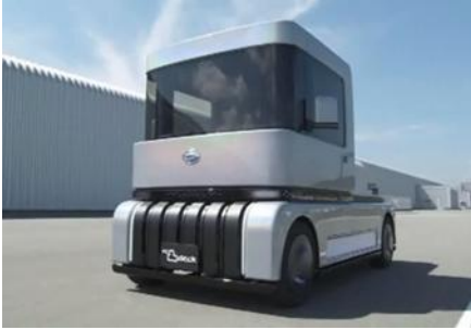
Fig. 1 Pt-free, zero-emission vehicle powered by a liquid-feed fuel cell.
